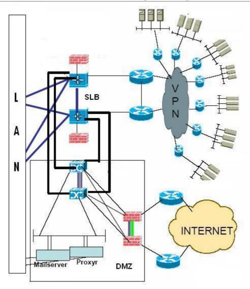
Operating offices are connected to data center using VPN. Requests from end-users will reach load-balancer from where they are routed to individual application servers. Mail & Proxy servers are in DMZ network. All the incoming traffic is screened by Firewalls. OHardware level redundancy exists.
